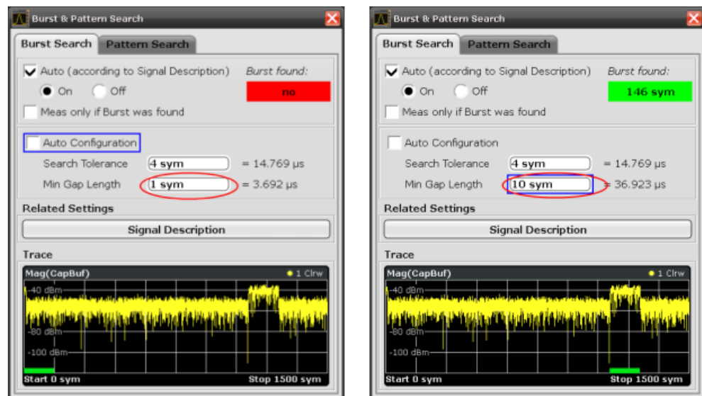
Fig. 4-91: Example for adjusting the minimum gap length
