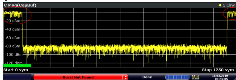
Fig. 4-87: Example for incomplete burst capture
